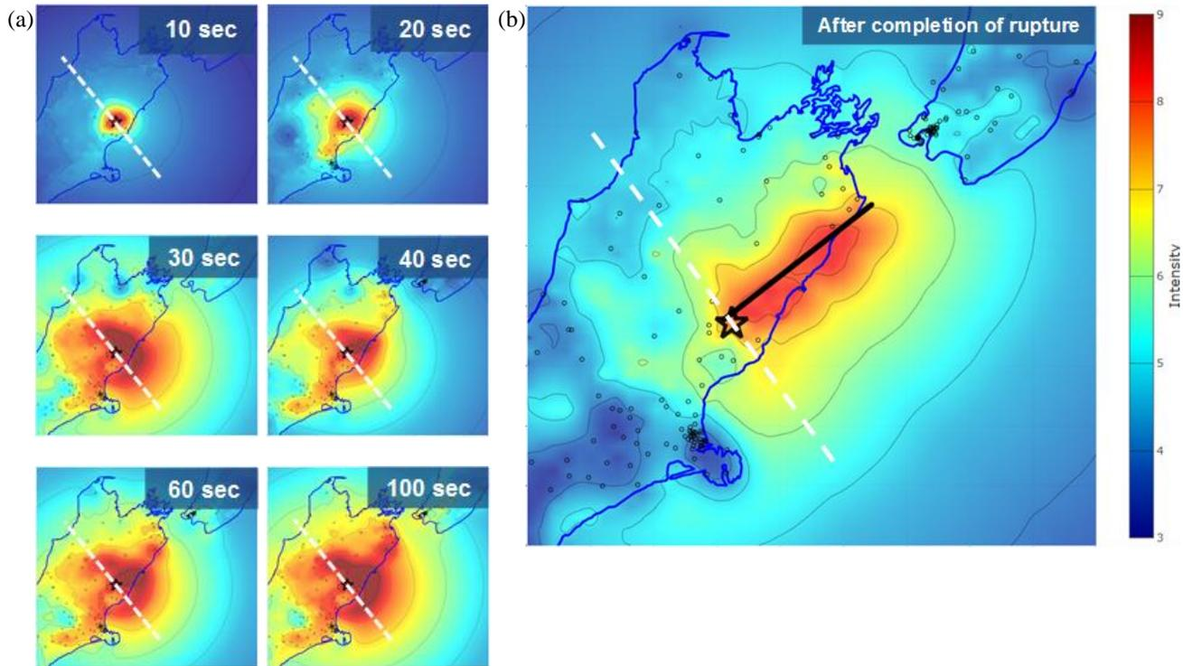
Figure 8. Evolution of the shaking intensity estimates based on assimilation of on-site predictions into regional GMPE predictions at a given time since the rupture initiation.
