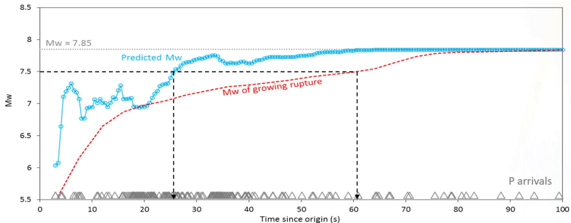
Figure 7. The evolution of  $M_w$  estimates based on Eqn (3) using  $P_a$  values measured from the entirety of the P-window that is captured up to a given point in time.
