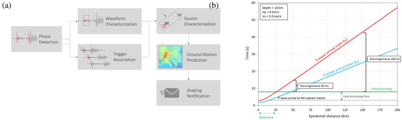
Figure 1. (a) General workflow for a typical EEW algorithm and (b) Seismic phase arrivals as a function of distance. Warning lead time is defined as the time difference between S-wave arrival (red line) and the initial warning (green line).
