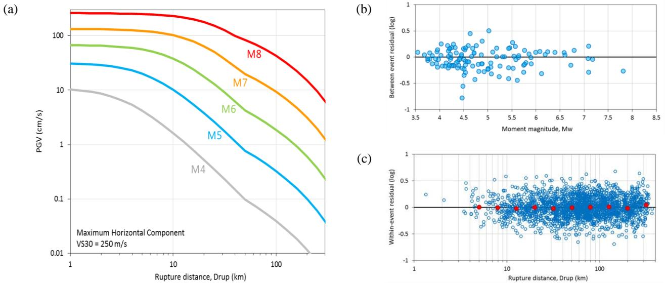
Figure 5. (a) The empirically calibrated generic ground motion prediction equation for New Zealand evaluated up to 300 km for  $M_w$  4 – 8 for a  $V_{S30}=250\text{m/s}$ . (b) Between-event residuals as a function of moment magnitude and (c) within-event residuals as a function of distance, where open blue circles show individual source, path and site corrected ground motion observations and closed red circles show logarithmically-spaced means.
