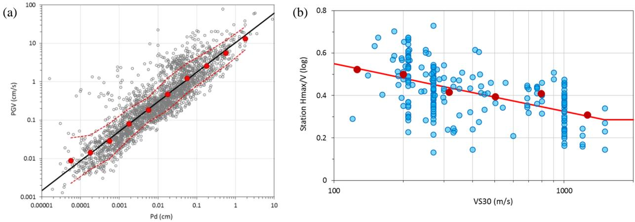
Figure 3. (a) Relationship between P-wave peak displacement ( $P_d$ ) and vertical peak ground velocity (PGV<sub>Z</sub>), where red circles show binned mean values, dashed red lines show one standard deviation around the means, and the solid black line is the model in Eqn (1). (b) Relationship between horizontal-to-vertical ground motion ratios and local shear-wave velocities ( $V_{S30}$ ), where red circles are the binned mean values and the red line shows the model in Eqn (2).
